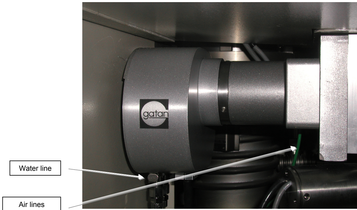
ORIUS™™ camera mounted on a TEM column.
