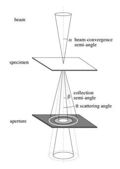
The angle of beam convergence is especially important when we are trying to illuminate an area on the specimen with a small probe. The angle for collection is adjusted with apertures or detectors to control the type and amount of image contrast, and has major influence on resolution (as we have seen). This is a
