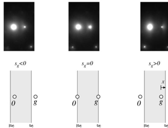
For small tilt angles, the relationship is linear. If the  $g$  line is offset from the reflection by a reciprocal-space distance  $x$ , the tilt from the zone axis is:
