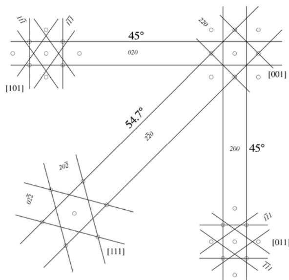
Apparently, if the  $g$  line passes on the other side of the  $g$  reflection,  $s_g > 0$ . In other words, the position of the  $g$  line relative to the  $g$  reflection provides a way to measure  $s_g$ .
