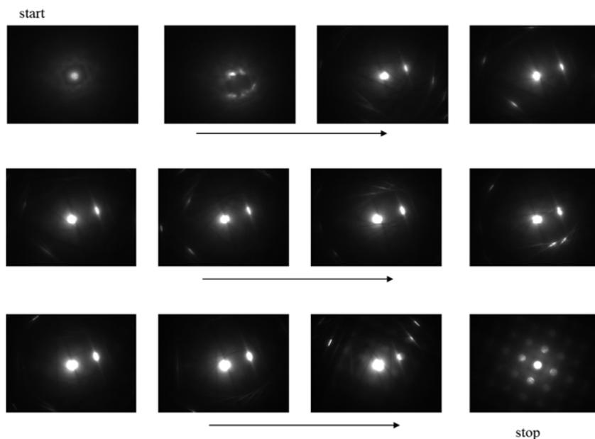
Note that, whereas we can see Kikuchi bands in selected-area diffraction patterns, they are even stronger in convergent-beam diffraction patterns, which we will discuss shortly. Some examples here use a convergent beam, rather than a parallel beam.
