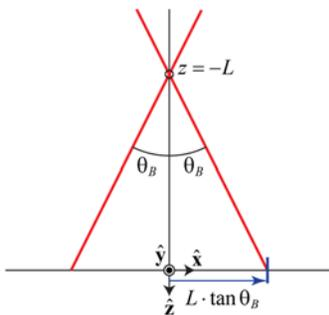
One thing to notice is that the Kossel cones tilt with the sample. We are not very concerned with the incident beam direction at this point, except to say that the diffuse scattering is strongest in the forward direction.
