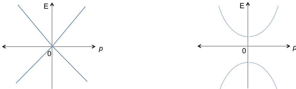
Figure 2: Energy E vs. momentum \mathbf{p} for (left): a massless particle and (right): a massive particle according to equations 4-5.
